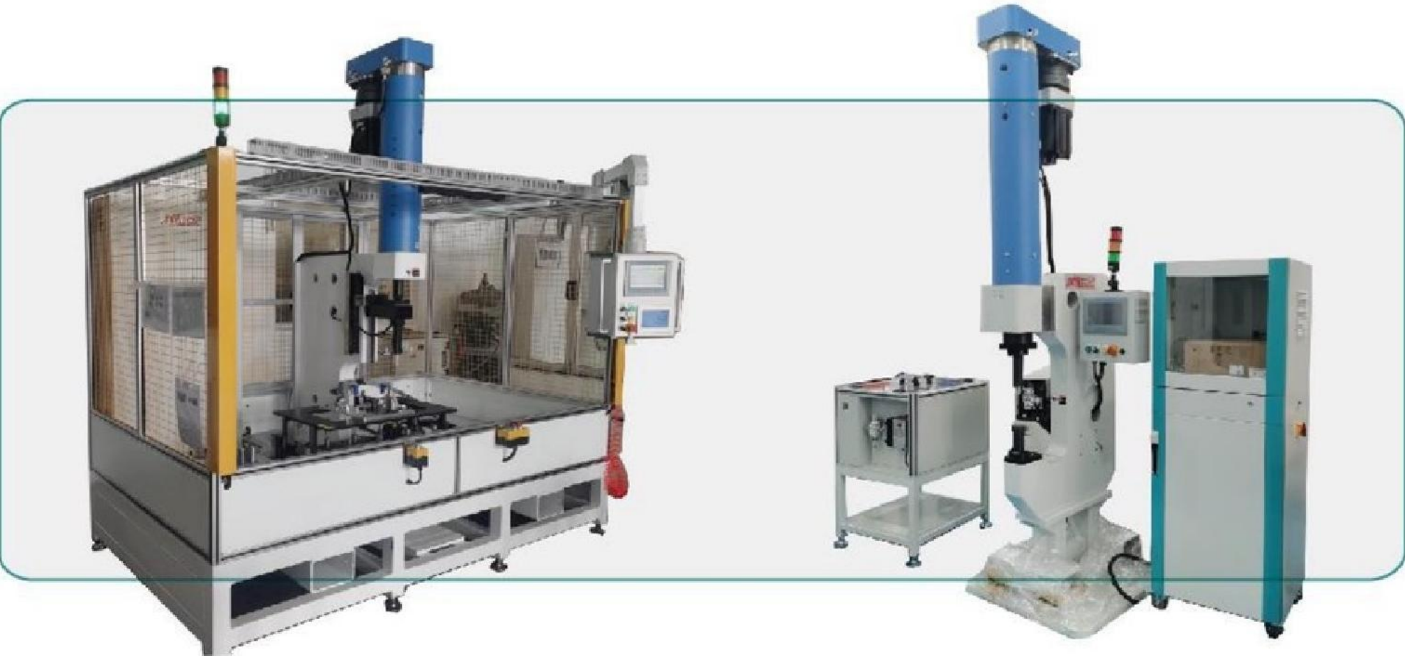
Intelligent riveting unit for sheet metal connection of new energy vehicles
